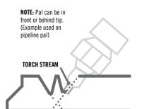
SET TORCH HEAD AT DESIRED 30 OR 33 **DEGREES AND LINE IT** UP WITH ADVANCED **CUT LINE OFF CENTRE** OF TORCH STREAM CLOSEST TO CRAWLER.
