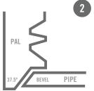
AFTER CUTTING THE PIPE, CHECK THE BEVEL WITH THE PAL
